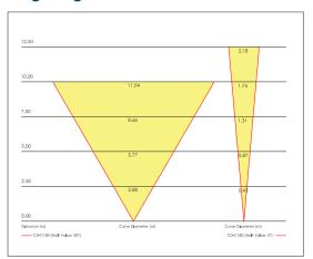
In lighting, choosing the lens angle is as important as selecting the color or wattage. Small angles retain brightness at long distances, while wide angles cover larger areas but lose brightness over distance.
